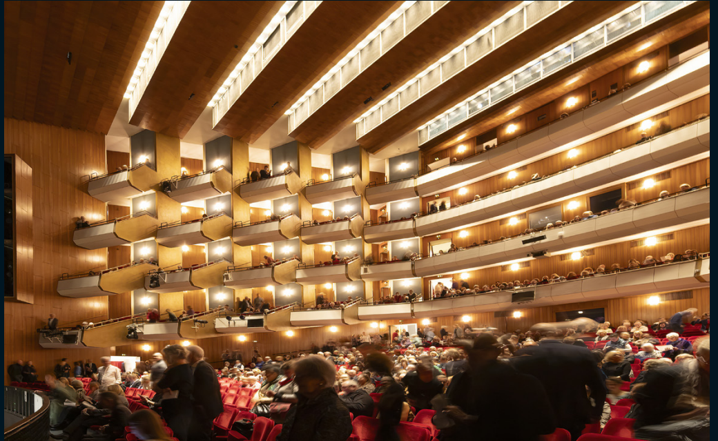
Hamburg State Opera, Hamburg For the refurbishment of the auditorium lighting, the opera house opted for customised Atrium double-focus downlight. The result: over 80% energy savings, excellent lighting quality and superior visual comfort. Lighting design: Ingenieurteam Gebäudetechnik GmbH & Co. KG Photography: Frieder Blicke
