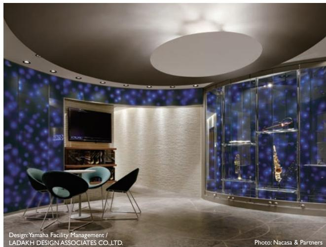
Kinetic cross-fading LEDs behind blue translucent panels create a striking display.
